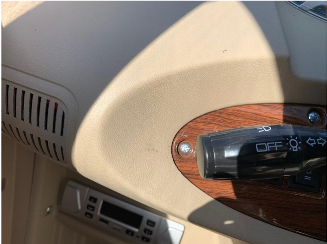
Blinker Arm and Light Control- Up is Right Down Is Left turn the knob from OFF to Light Icon to turn on head lights
